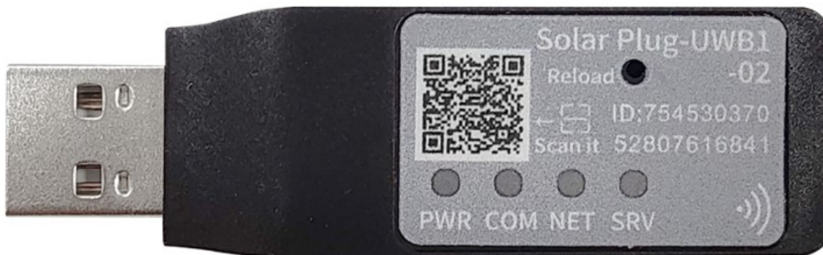
Figure 3. 产品正面指示灯和重置按键
