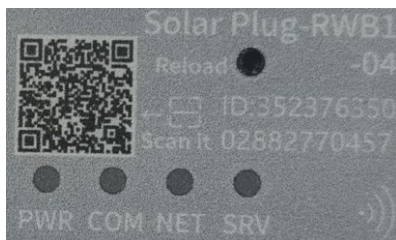
Figure 4. 产品正面指示灯和重置按键
