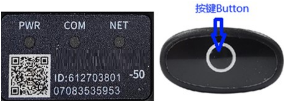
Figure 4. 产品正面指示灯和重置按键
