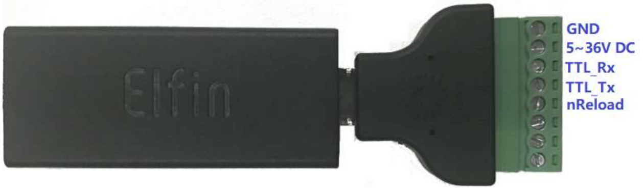
Figure 9. Solar Elf-SEW42B+8PIN 端子
