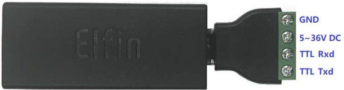
Figure 13. Solar Elf-SEW42B+4PIN 端子
