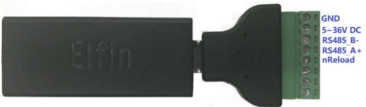
Figure 8. Solar Elf-SEW41B+8PIN 端子
