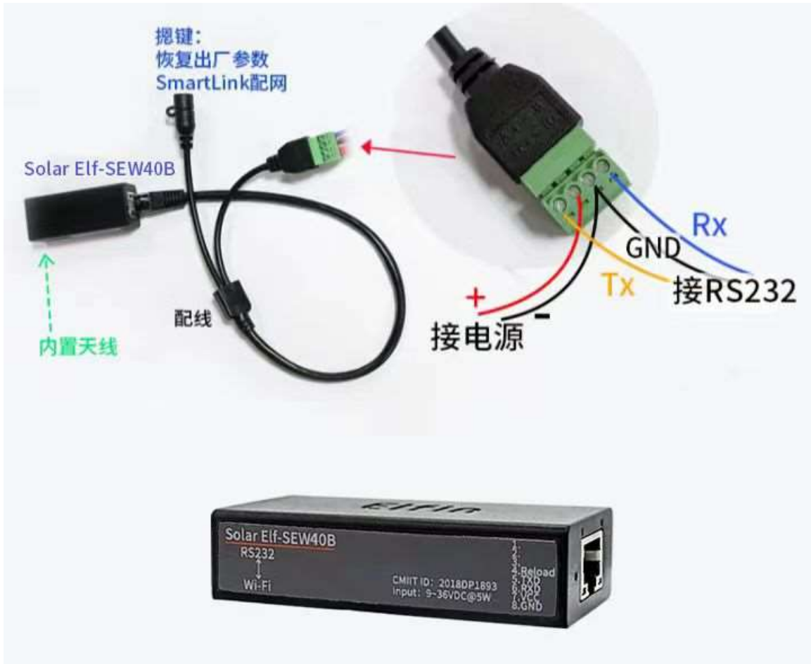
Figure 15. Solar Elf-SEW40B+RJ45 转换线缆
