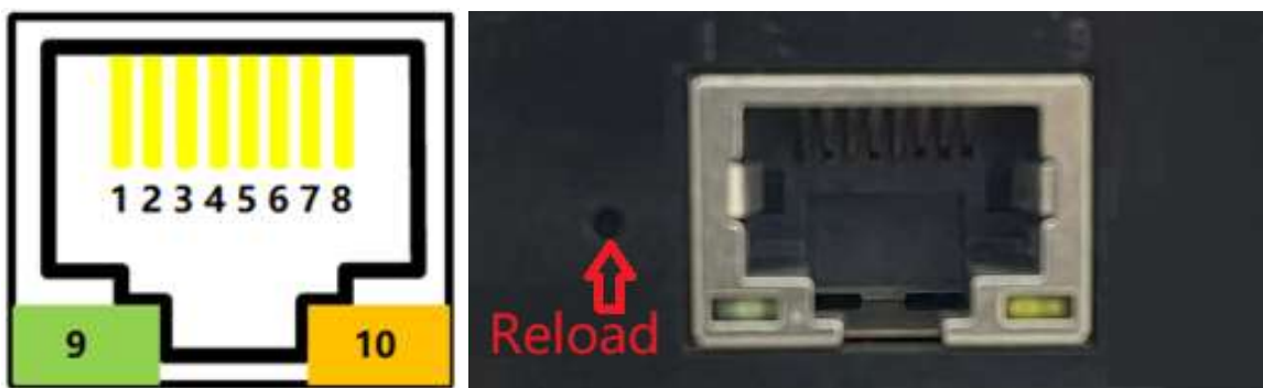
Figure 4. RJ45 引脚标号
