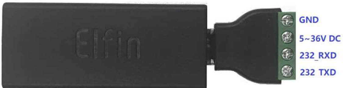
Figure 11. Solar Elf-SEW40B+4PIN 端子
