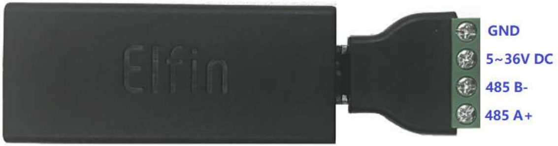
Figure 12. Solar Elf-SEW41B+4PIN 端子
