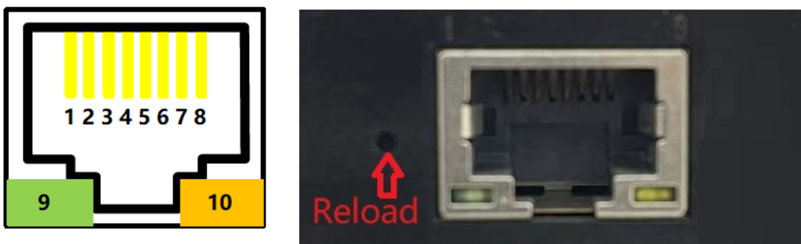
Figure 6. Solar Elf-SEG4xB RJ45 接口引脚定义
