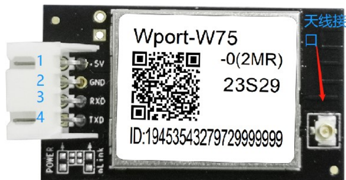
Figure 3. Wport-W75-X(2MR) Pin Definition
