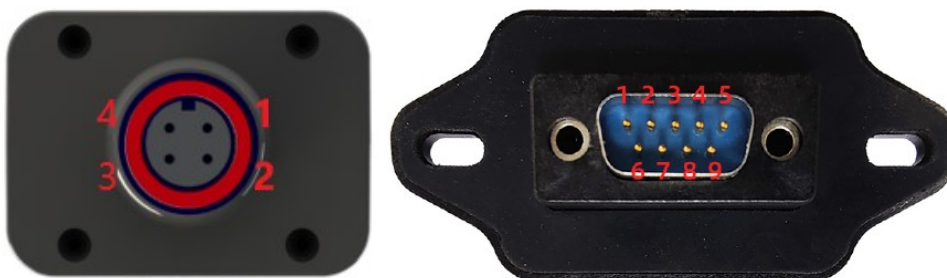
Figure 10. Pin Markings Of The Red Aircraft Female Head And DB9
