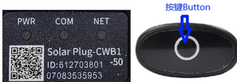
Figure 4. Front indicator Light and Reset Button Of The Product
