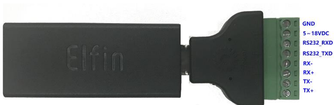
Figure 7. RJ45 8PIN 端子
