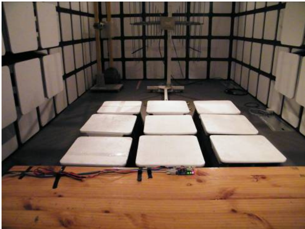
Picture 6 RF Electromagnetic Field (RS) Test Setup
