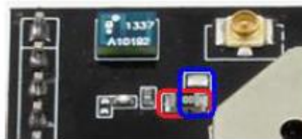
Figure 6. Exchange Resistor between Internal and External Antenna
