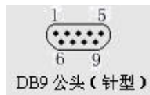
Figure 4. RS232 Pin Defination(Male/Needle Type)
