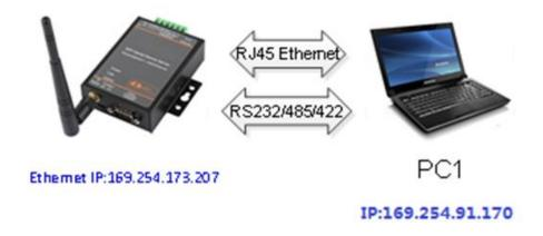
Step 1: Ethernet cable connects RJ45 ports between device and PC. Open IOTService and it will achieve device information automatically. Figure is as below:
