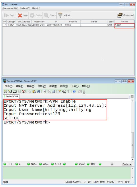
Step 5 : VPN test address is 192.168.18.1, and following figure represents successful connection.
