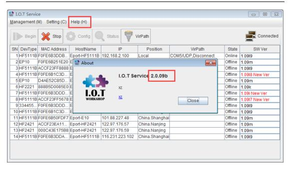
Step 3: Wireless connection between serial device and PC WiFi. Open IOTService and copy mac address of serial device. It will be used in step 7.
