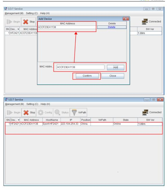
Step 8: Edit device and create virtual serial port. Only UDP connection supported.
