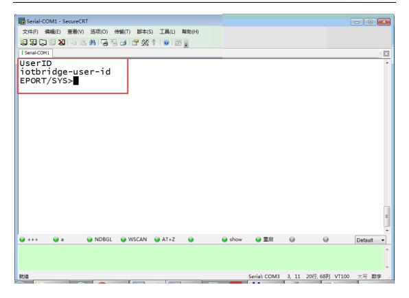
Step 6 : Set server address and type "+++" to enter cmd mode->SYS->NAT Enable-> input server address(same as IOTService) -> set port(default is ok)-> SET-OK. Specific can refer following setting.
