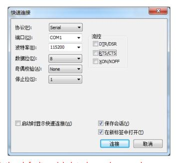
Notes: HF2421 the default serial data is as above and user can modify device working parameter by IOTService.
