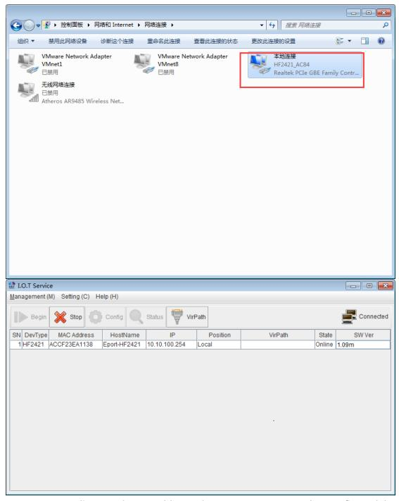
Step 2 : According to the IP address above, parameter can be configured by webpage. Username and password are both admin as default.
