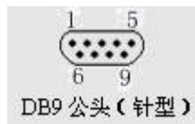
Figure 3. RS232 Pin Defination(Male/Needle Type)
