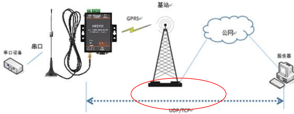
Figure 5. GPRS wireless network
