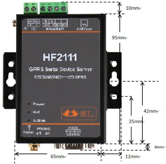
Figure 4. HF2111 机械尺寸
