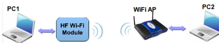
Figure 24. STA Interface Debug Connection
