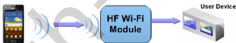
Figure 28. Wireless Control Application
