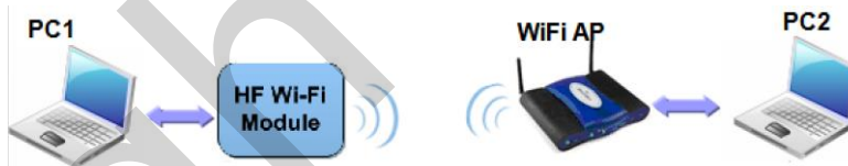
Figure 22. STA Interface Debug Connection
