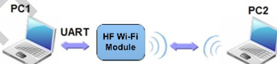
Figure 23. AP Interface Debug Connection
