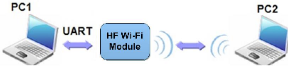
Figure 25. AP 接口连接调试
