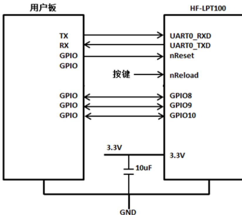
Figure 6. HF-LPT100 UART 应用硬件连接
